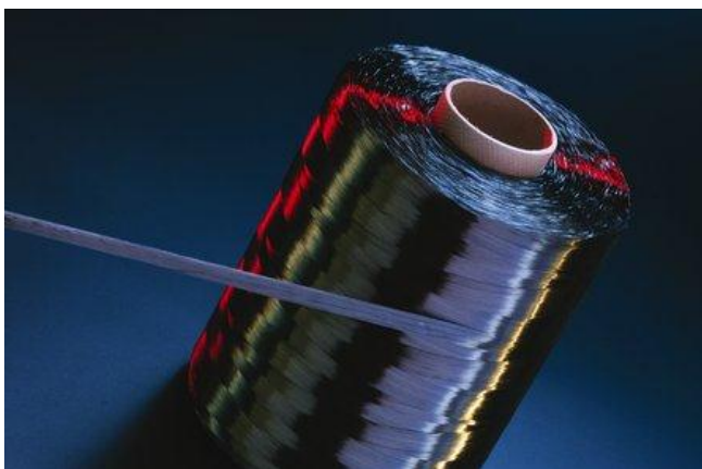
Fig. 1: Bundle of 50000 carbon fibers (Image: SGL Group)
