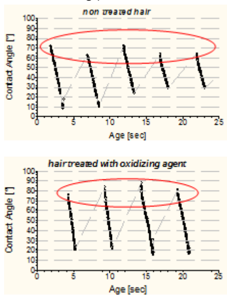
Picture 5: Contact angle measuring data of five water drops of approx. 100 pl applied at intervals of 5 s, on non-treated hair (above) and of four water drops of approx. 100 pl on hair treated with oxidizing agent in dependency of the total measuring period. The image acquisition speed of the camera was 250 fps.
