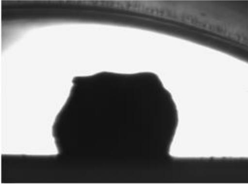
Fig. 10: Slag on Al<sub>2</sub>O<sub>3</sub> at approx. 1365°C
