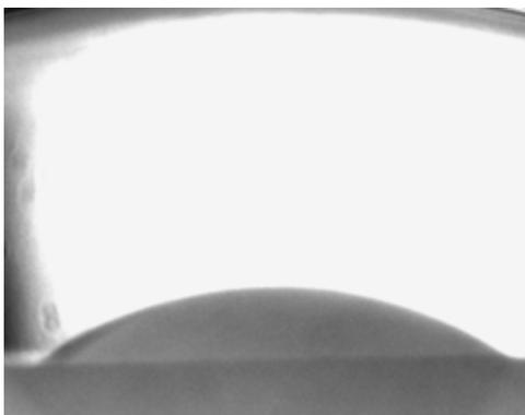
Fig. 7: Molten slag on graphite at approx. 1700°C
