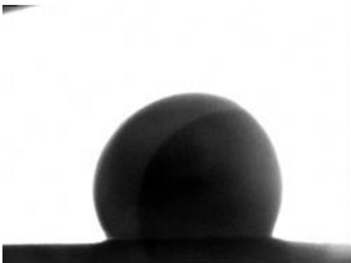
Fig. 5: Slag sample on graphite at approx. 1635°C
