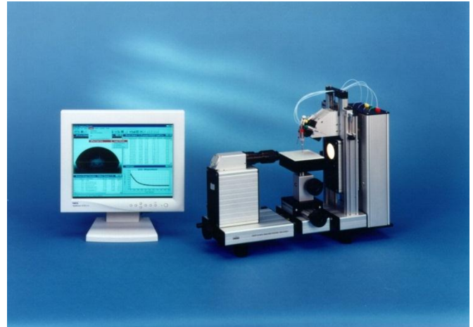
Figure 1: Drop Shape Analysis System DSA10DO4 from KRÜSS GmbH
