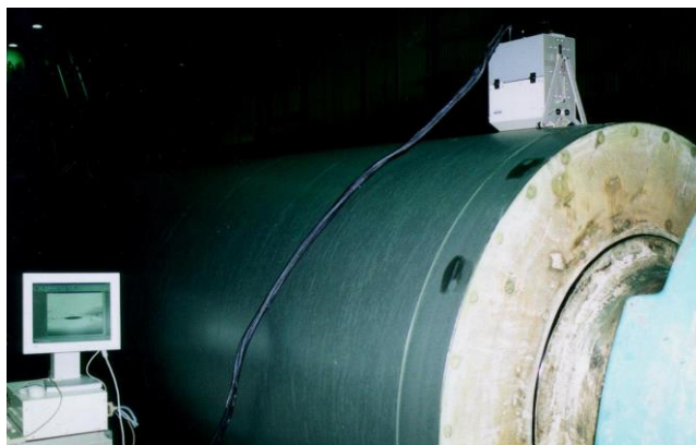
Fig. 3: GH100 being using for testing a printing roller at a production location.
