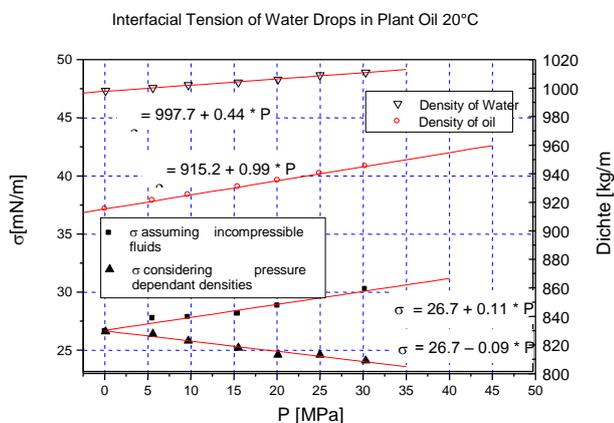
Fig. 6: Interfacial tension as a function of pressure
