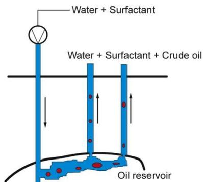
Fig. 2: Diagram showing tertiary oil recovery
