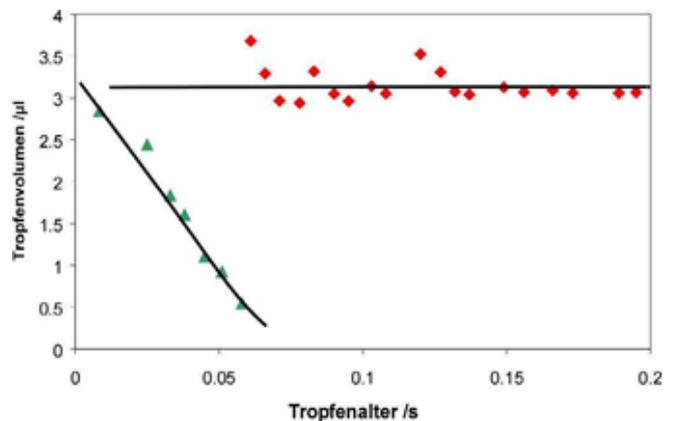
Fig. 3: Drop volume in dependence of drop age. Red squares: sample barely absorbent; green triangles: sample highly absorbent.
