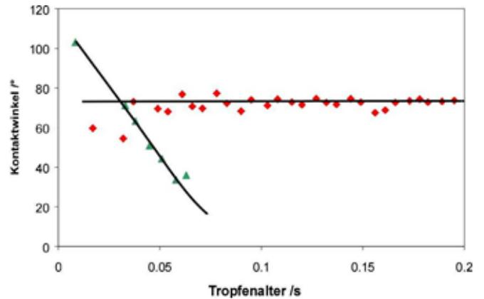
Fig. 2: Contact angle in dependence of drop age. Red squares: sample barely absorbent; green triangles: sample highly absorbent.
