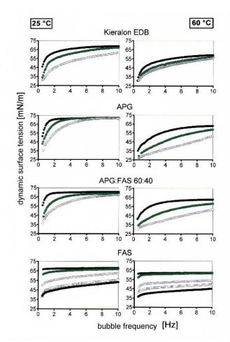
Fig. 2: Dynamic Surface Tension vs. Bubble Formation Frequency at various surfactant concentrations and temperatures. Surfactant concentrations:
