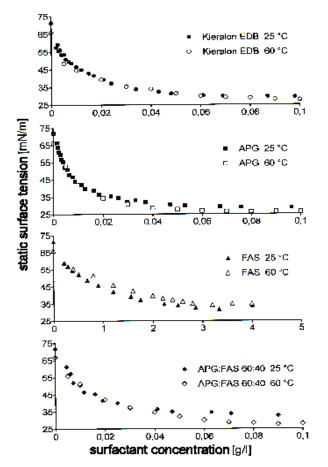
Fig. 1: Static surface tension of surfactants and mixtures depending on concentration and temperature
