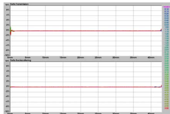
Figure 8. Transmission (top) and backscattering (bottom) for formulation 1 at 25°C.
