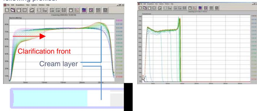
We can observe very easily on the left graph that the backscattering flux decreases at the bottom of the sample due to a decrease of the concentration of the particles in this part (clarification) and it increases at the top of the sample due to an increase of the concentration of the dispersed phase (creaming). Creaming can lead to a phase separation, with a clear phase at the bottom shown by a peak in transmission (right graph).
